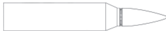
FIG. 475. 7.62mm Caseless Cartridge with Molded IMR Propellant and M59 Ball Bullet (from specimen).
