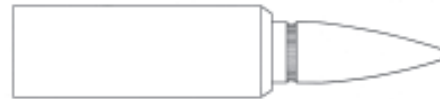
FIG. 481. 7.62mm Caseless Cartridge from Lot C-1 with M80 Ball Bullet (from specimen).
