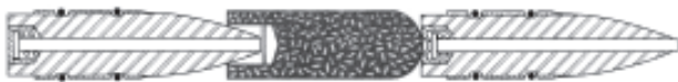
FIG. 474. 7.62mm “Bulpin” Test Device Cartridge Assembly (from Fig. 4, FA Rept. R-1750, Jan. 1965 and specimens).
