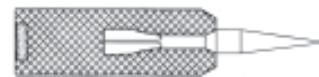
FIG. 435. Cal. .125 Caseless Flechette Cartridge FAT 143 (Fincon) (from FA Tech Rept. R-1696, Fig. 2, Sept. 1963).
